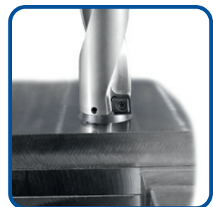
Paketbohren Bundle drilling
