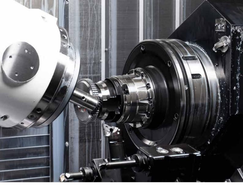
Prior to the introduction of the gear skiving process, the components were being manufactured with conventional cutting tools. "We were in the process of reorganising the production of our families of gears", explains Pascal Moulènes. With the help of the new technology, Moulènes was able to optimise the production processes because fewer set-up operations were required and he also managed to eliminate the idle time between work
