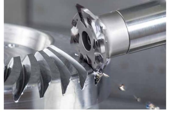
For sizes ranging from module 4 to 30, HORN offers gear cutting solutions for prototypes and small and medium-sized series on universal machining centres.
