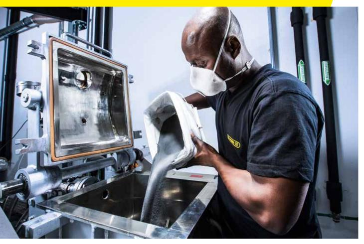
The manufacturing process for an insert starts with mixing and preparing carbide alloys in powder form.
