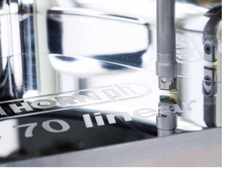
Mirror finish over the entire surface. HORN and DMG MORI use a sine wave to demonstrate their expertise in brilliant-finish machining of aluminium.
