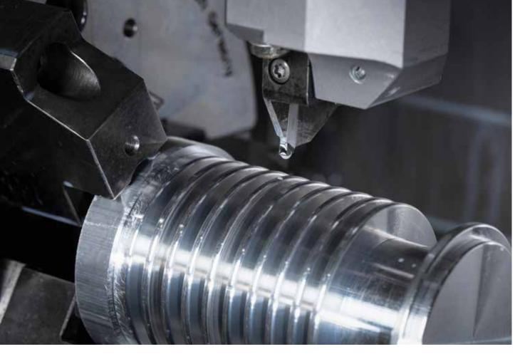
Aluminium cooling fins were to be cut for a pump in a medical device – a challenge that had to be mastered reliably with the right tools and expertise.
