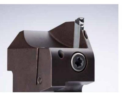
The polished WA chipbreaker geometry enabled problems of long chips and built-up edges during aluminium machining to be resolved.
