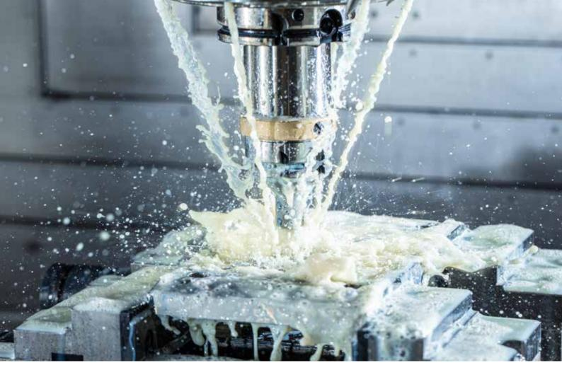
HORN has developed a set of speed-forming tools for machining grooves into cubic workpieces with maximum productivity.
