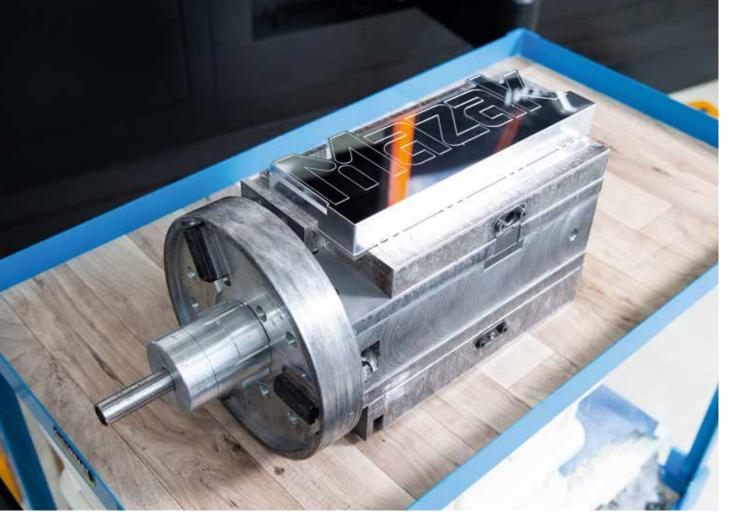
The solid workholding attachment developed by Mazak.
