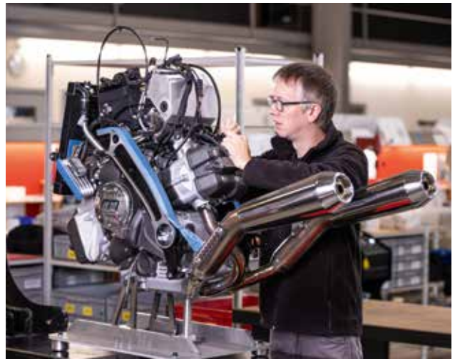
Great care is taken during final assembly of a Midual Type 1.
