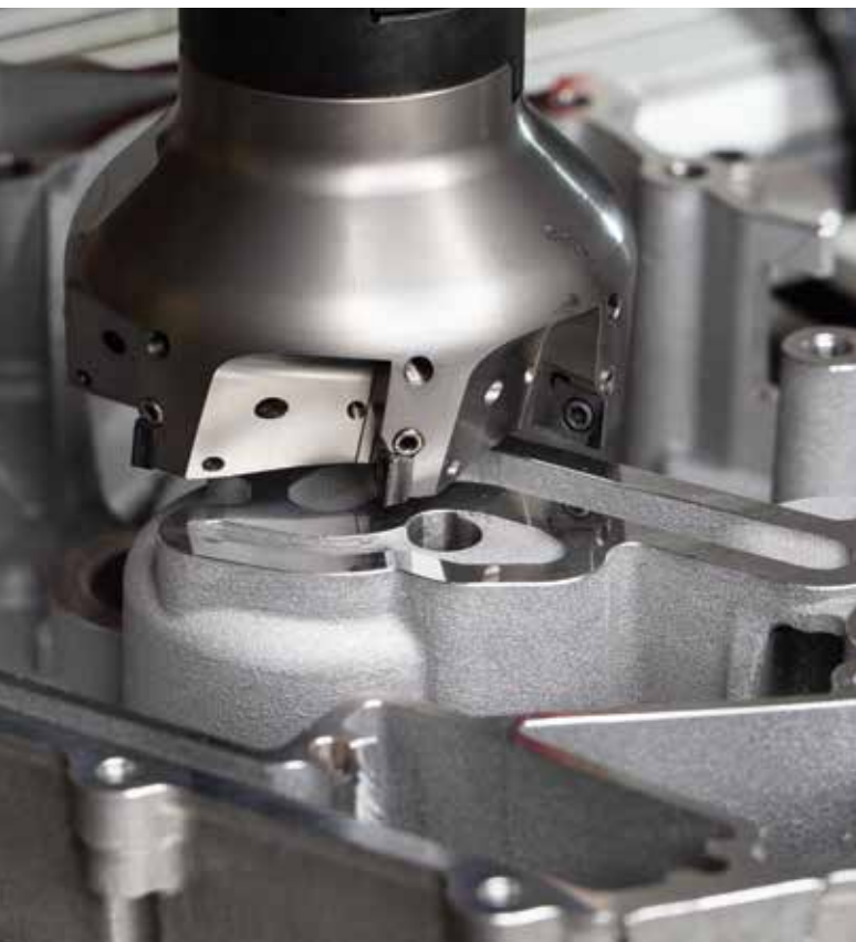
The HORN DTM milling system with PCD inserts ensures high surface quality on the aluminium components.
