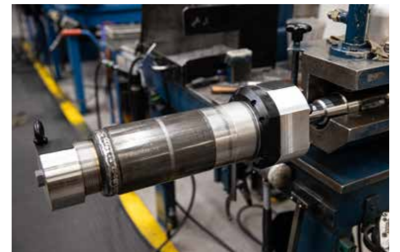
Assembly of the hydraulic cylinder used in the moving floor systems.
