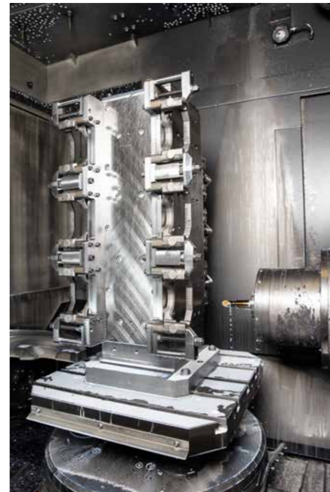
14 blanks are clamped onto a tower for machining.
