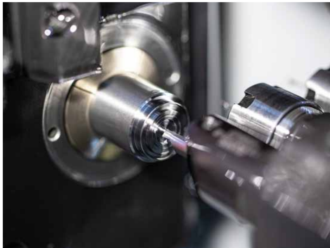
Face grooving of the medical component with the Supermini 105 system.
