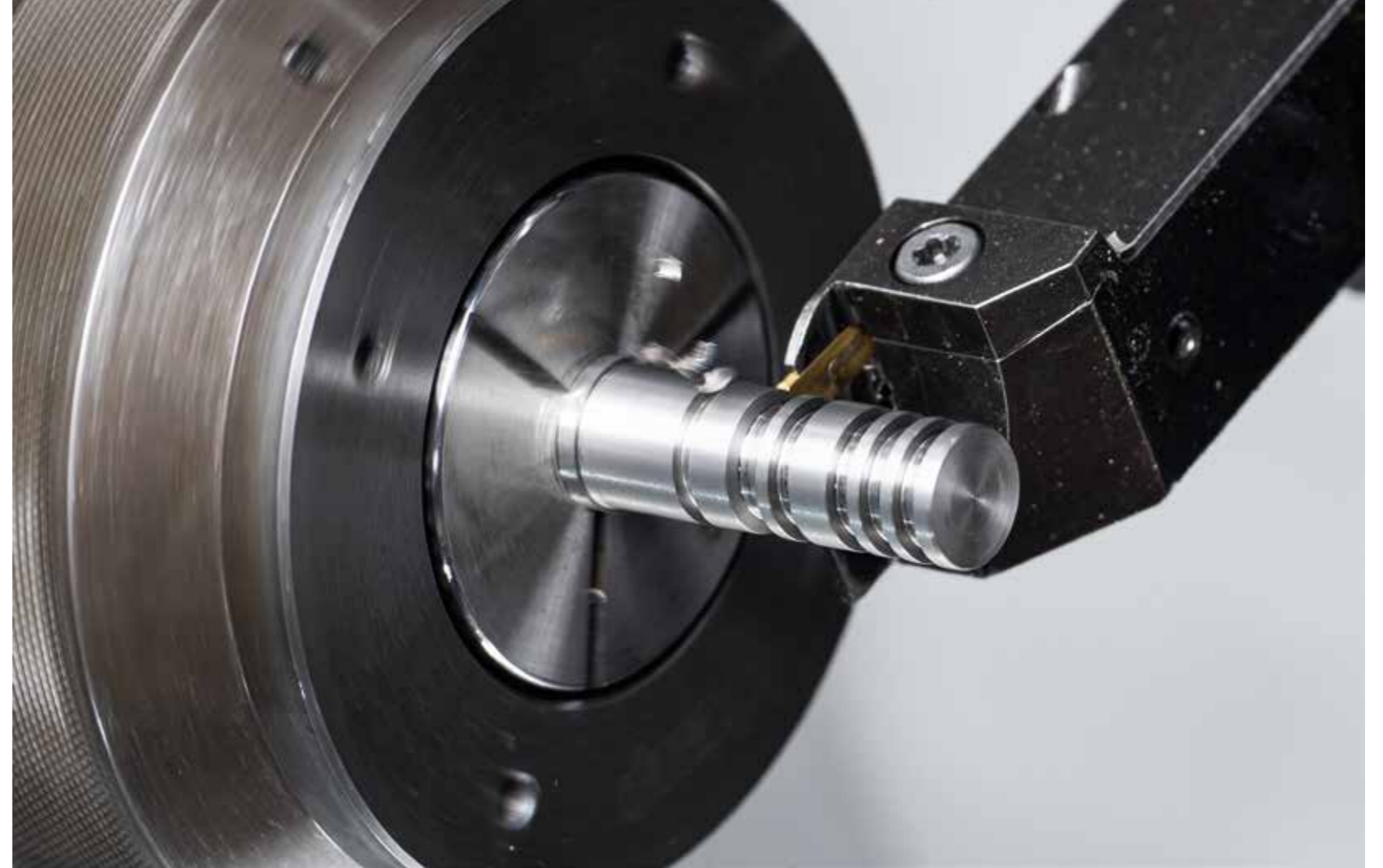
Minimum quantity lubrication enables higher cutting speeds than dry machining and also results in a better surface finish.
