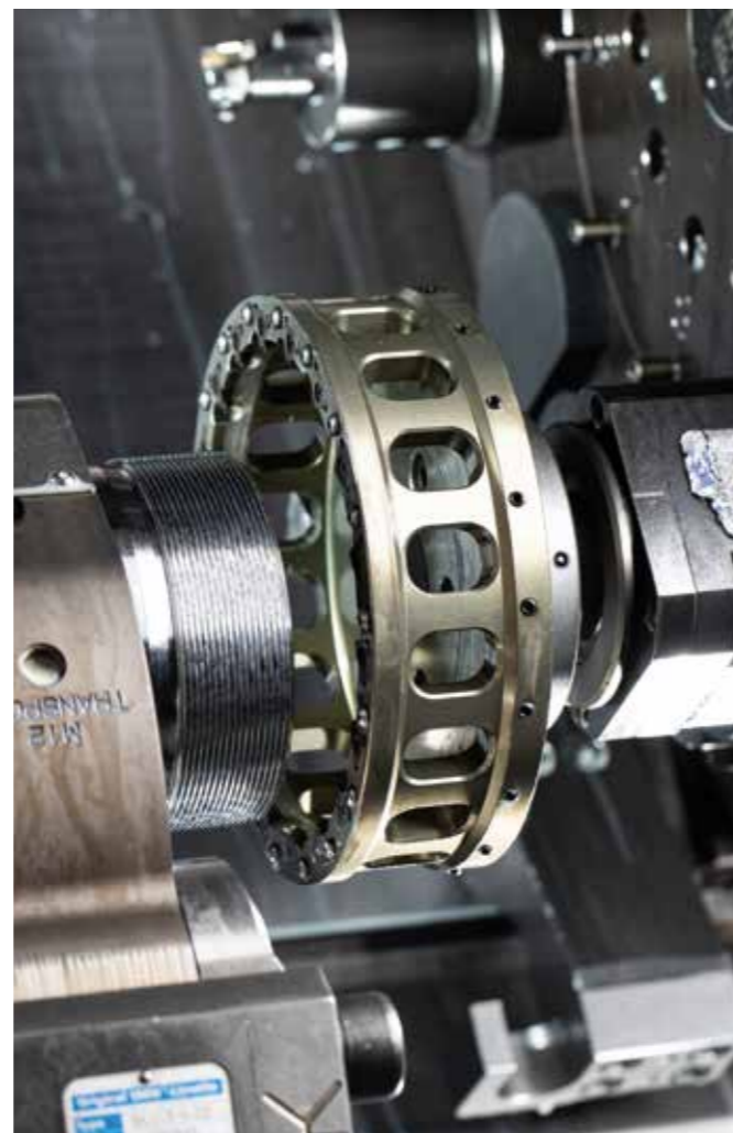
The changeover to the shell mill resulted in a large time saving and increased process reliability.
