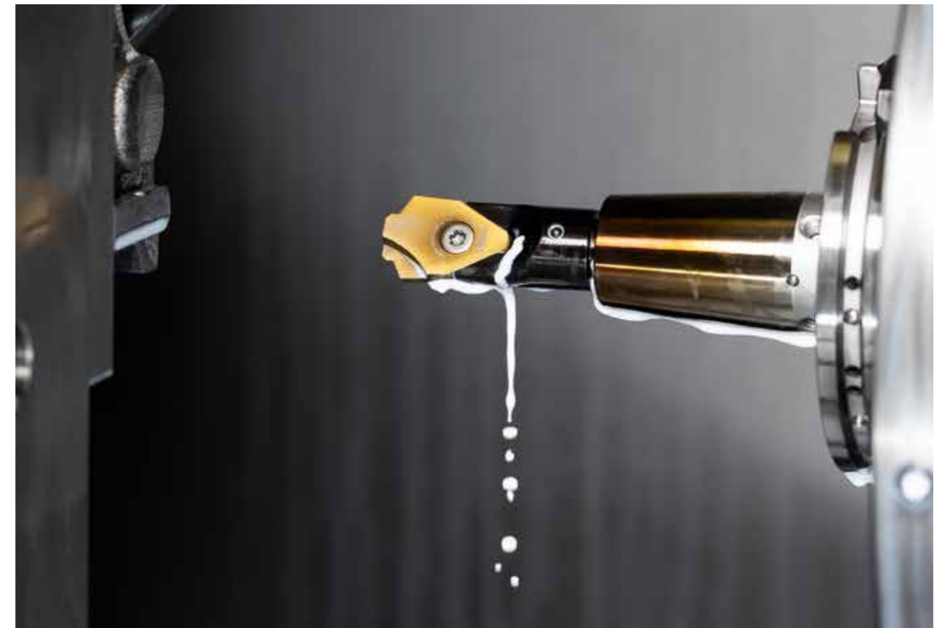
HORN's D117 form drilling tool produces the hole profile in one operation.
