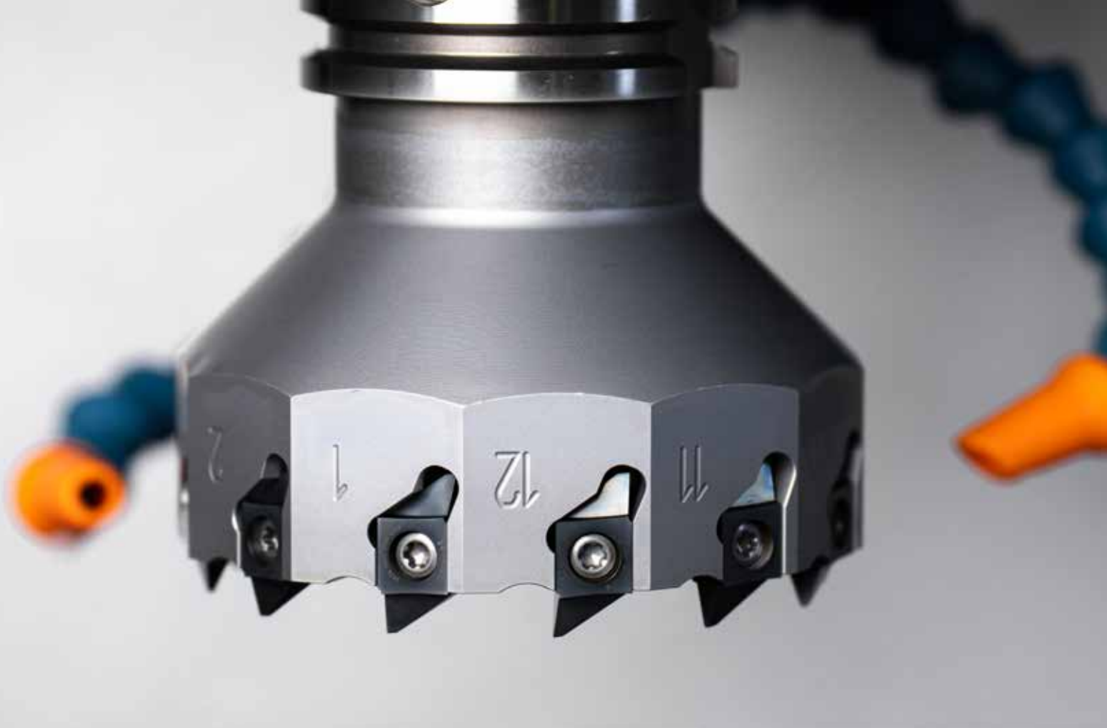
3.5 inch diameter cutter with 12 insert positions; inserts customised for EMCO's tooth form.
