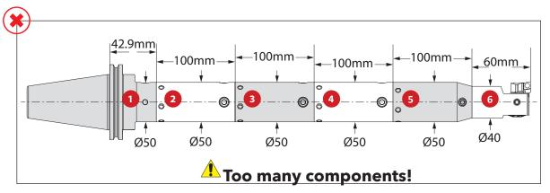
**NOTE**: Length to diameter ratio is calculated using body diameters, not cutting diameter.
